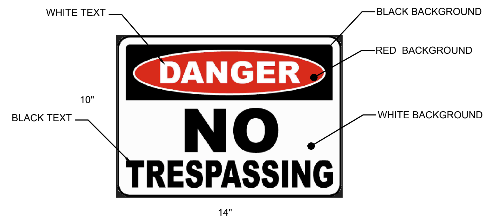
RED/WHITE/BLACK BACKGROUND, BLACK/WHITE LETTERING MOUNTING LOCATION: ACCESS GATE QUANTITY: 1
