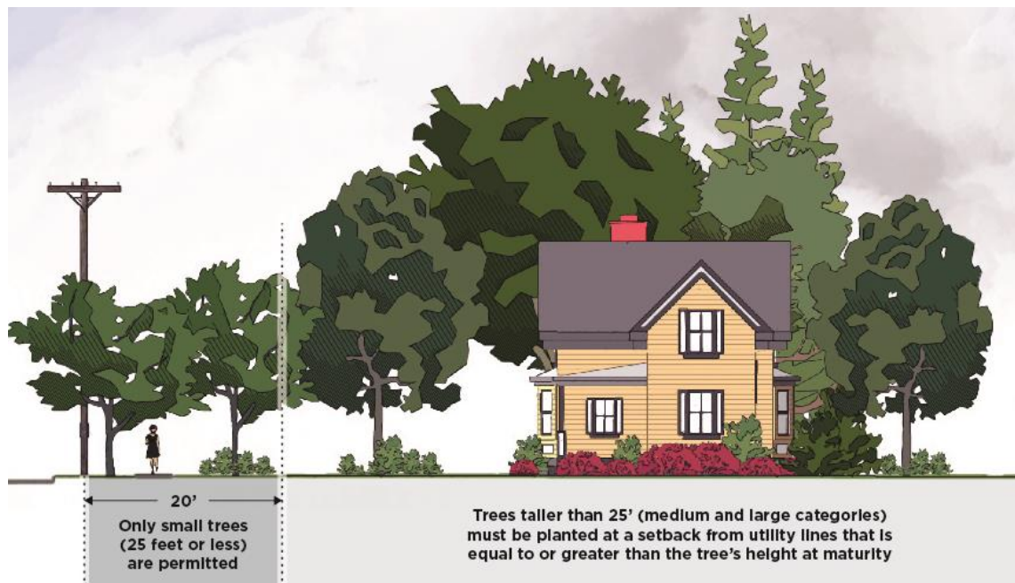
FIGURE 10-1: OVERHEAD UTILITY PLANTING ZONES
